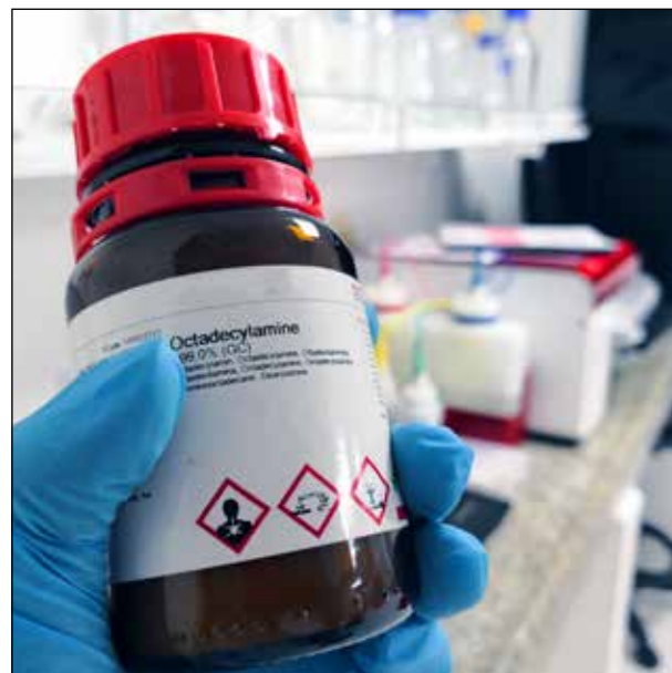
2-color labeling for hazardous warnings
